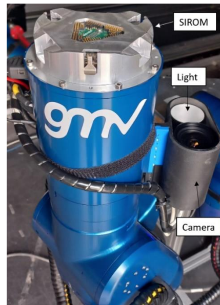
Figure 4: Camera, light, and end-effector SIROM in one of the manipulator arms.
