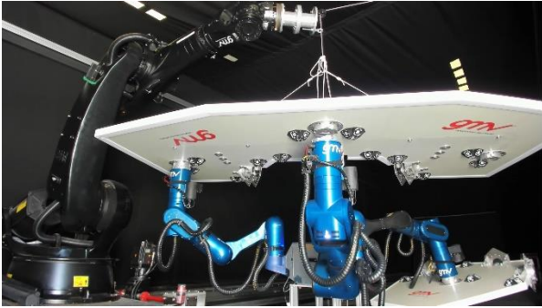
Figure 9: Test setup in the platform-art testing facility, with the multi-arm manipulator attached to the spacecraft mockup and manipulating a SMT for assembling it.
